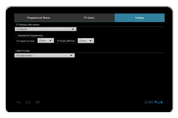
Settings Tab: This tab will control the settings of the app. It will be capable of selecting the TV brand, the cable provider, and what times the TV will turn on and off each day.
