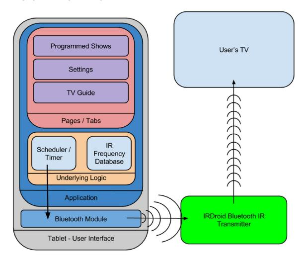
Our system is built around android development, and the open source device known as the IRDroid v2.0 Bluetooth IR transmitter. Our application will be run on an android device and contain two main components.
